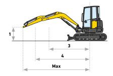
The lifting capacity is based on the ISO 10567 and it does not exceed more than the 75% of static tipping load or more than the 87% of the hydraulic lifting capacity of the machine.
