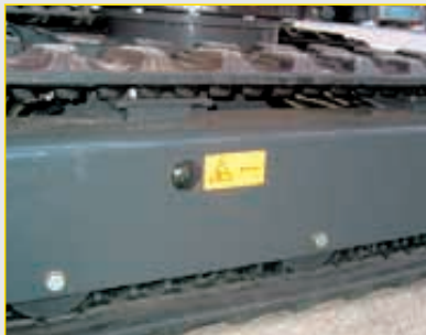
Simple track tension adjustment with grease pump.
